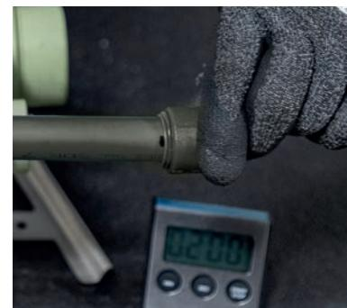
When the pipe and the fitting are welded, their plastic materials fuse together to form a homogeneous, firmly bonded whole. Special tools are used to heat up pipe and fitting, which are then just joined together. This connection is reliable and lastingly leakproof.
